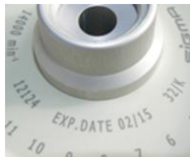
Fig. 2: Different service life – engraving on the bucket/rotor
