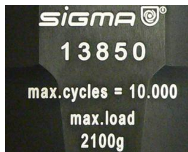
Fig. 2: Different service life – engraving on the bucket/rotor
