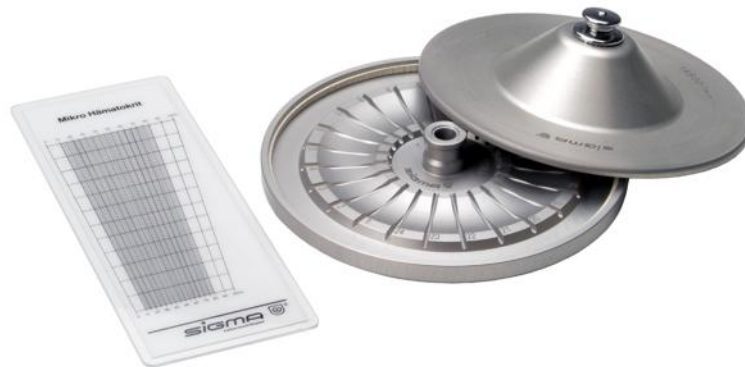
Fig. 7: Microhaematokrit rotor (part no. 11026) with reader (part no. 17028)
