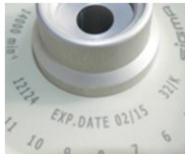
Fig. 4: Different service life – engraving on the bucket/rotor
