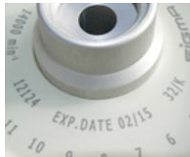
Fig. 7: Different service life – engraving on the bucket/rotor
