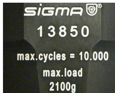
Fig. 7: Different service life – engraving on the bucket/rotor
