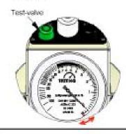
10. Screw down the threaded tube onto the left ball shut-off valve. Let the tube hang into a suitable graduated cylinder and open the ball shut-off valve. Operate the TEST valve and pump with the hand pump until 100 ml (1-litre unit), 250 ml (5-litre unit), or 400 ml(8-litre unit) of water has flowed out. Then close theleft ball shutoff valve.
