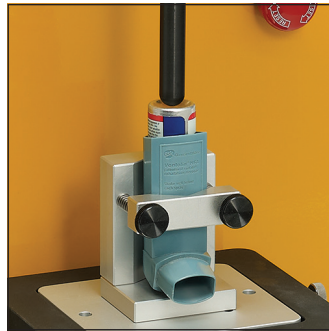
TA-MDI P Metered Dose Inhaler Fixture measures the push-button force to actuate the inhaler. Fixture Base Table required.
