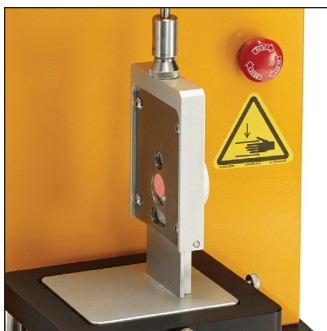
TA-BLS P Bi-Layer Shear Fixture measures shear strength by cutting a two-part tablet or capsule using a guillotine blade. Fixture Base Table required.
