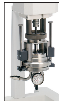
RST-90Y Spindle for BU measurements on joint compound and similar materials
