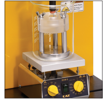
TA-MA P Muco Adhesion Test Fixture Simulates body/temperature conditions and force needed to pull a tablet away from a mucosal surface.
