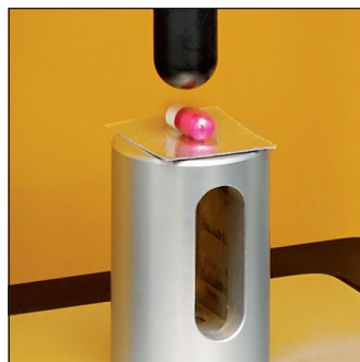
TA-BPS P Blister Pack Support Fixture is used to measure the force required to remove the tablet from its blister pack. Fixture Base Table required.
