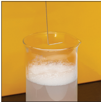
TA-RT P Raft Tester measures alginate Raft Strength by pulling wire raft hook out of the sample material.
