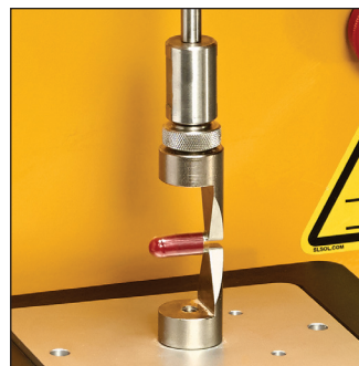
TA-CLT P Capsule Loop Tensile Test Fixture is used to measure the force required to split one half of a hard gel capsule. Fixture Base Table required.
