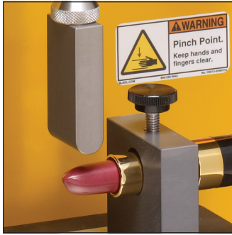
TA-LC C Lipstick Cantilever Test Fixture allows imitative tests on lipstick and similar products to quantify strength of product. Fixture Base Table required.
