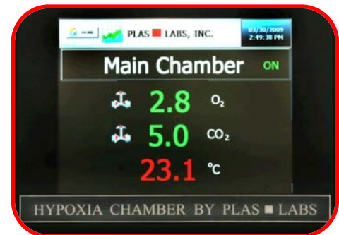
Main “Touch Screen” control panel
