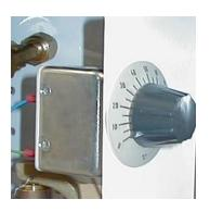
Typical View of Cooling Lock Thermostat
