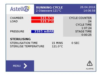
This stage is the main sterilisation process. The stage timing is controlled by the selected temperature probes and the temperature by the pressure set-point. The stage continues for set sterilisation time.
