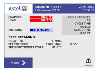
The chamber temperature will stabilise and slowly rise typically 97-103°C depending on altitude and the boiling point of water. After free steam time ends, the system goes to heat to sterilize stage.
