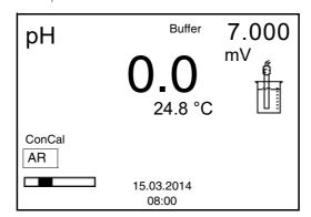
Wait for the end of the measurement with stability control or accept the calibration value with **<ENTER>**.
