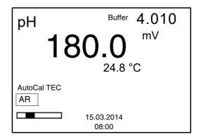
19 Wait for the measurement with stability control to be completed or terminate the stability control and take over the calibration value with **<ENTER>**.
