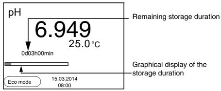
The active automatic data storage function can be recognized by the progress bar in the status line. The progress bar indicates the remaining storage duration.
