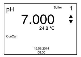
Set the nominal buffer value for the measured temperature with <▲ ><▼ >.
