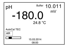
Wait for the end of the measurement with stability control or accept the calibration value with **<ENTER>**. The calibration display for the next buffer appears (voltage display).
